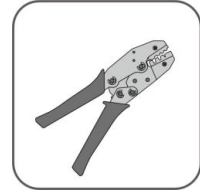
Tube terminal crimping tool (0.5 mm 2 –1.0 mm 2 )
